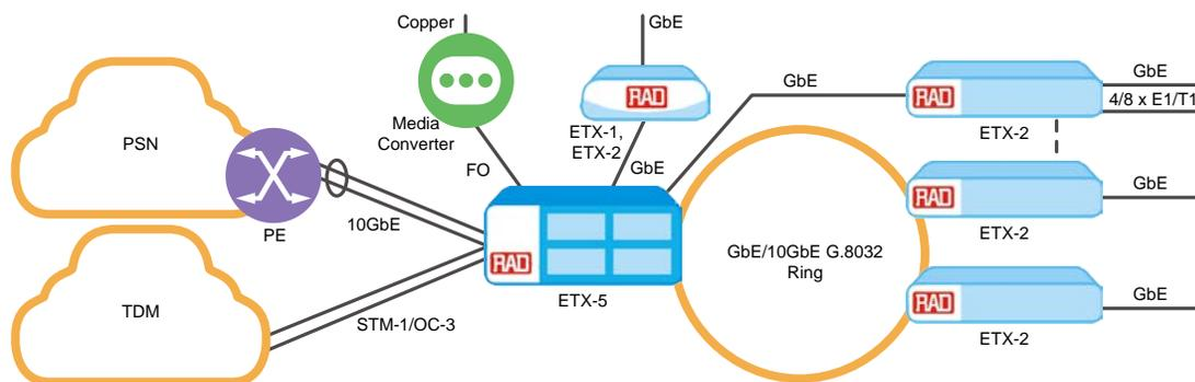
Figure 1. Access Aggregation with SLA-Based Services
